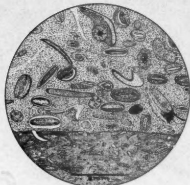
FIGURE 2. ODD-SHAPED FOSSIL FRAGMENTS ORIENTED PARALLEL TO BEDDING Covered with radially growing carbonate. Ooids are few and irregularly distributed. Rose Hill (Silurian), Md. Lower McKenzie.
